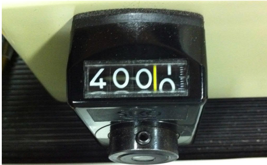
Figure 4. Correct reading of the DM150 wavelength indicator after driving the monochromator to 400 nm.
