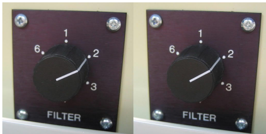
Figure 3. Filter wheel knob position. Correct position (left) and wrong position (right).
