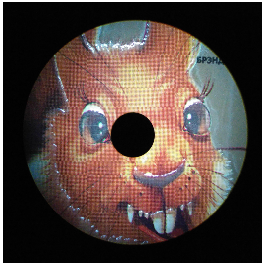
Figure 3: View of the viewfinder. Black circle in the middle corresponds to the 1^\circ measurement spot.
