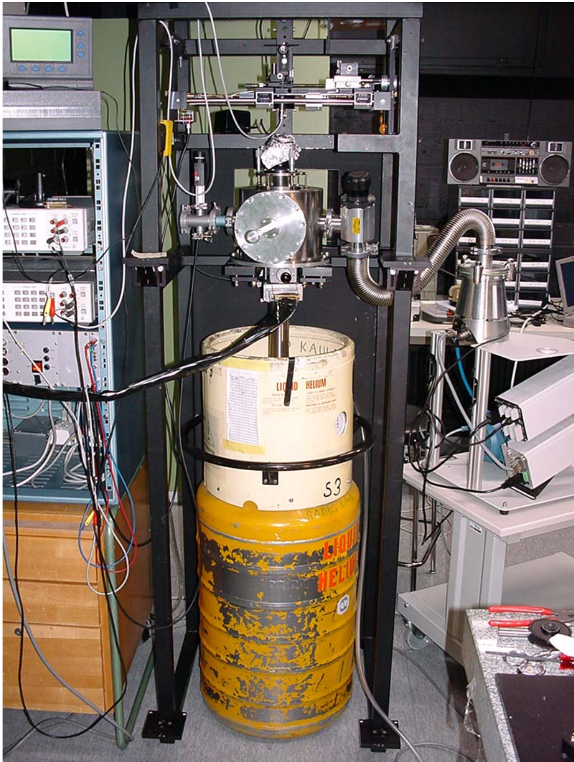
Figure 4.11. Cryogenic radiometer in the measurement setup. The entrance window should remain covered whenever measurements are not conducted.
