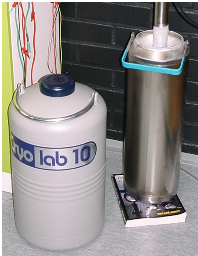
Figure 4.9. Cryo in Nitrogen. There should be a rag around the cryo cavity to reduce the ice formation. It was forgotten during the 2003 measurement session.
