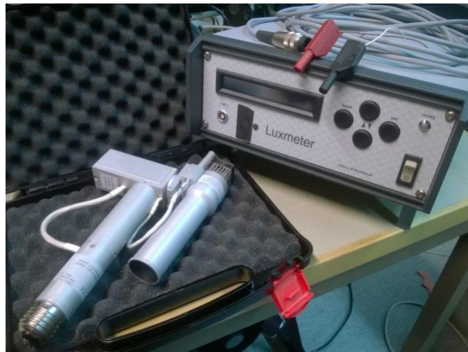
Figure 4. Czibula & Grundmann Sphere scanner, the control unit and the cable to connect them to each other.
