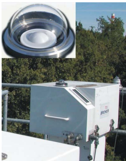
Figure 1. Brewer MKIII #163 with the global input optic for measuring spectral UV irradiance. The first optic was installed in 2002. It was replaced in 2004 by the new and further improved global input optic. Courtesy J. Gröbner, JRC, Ispra.
